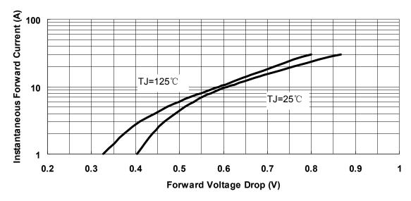
Fig.3-Typical Instantaneous Forward Voltage Characteristics
